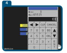
A keypad will pop up. Use the keypad to enter the full scale value of your transducer and press enter. The configuration screen will return with your value in the "Pressure at 20mA" field. You can also enter a value other than zero for the smallest value to be displayed, and you can enter a value for the display increments (factory set at 1).
