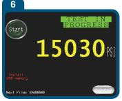
When the test is complete, press the light green "Stop" button. This will stop the data logging process.
